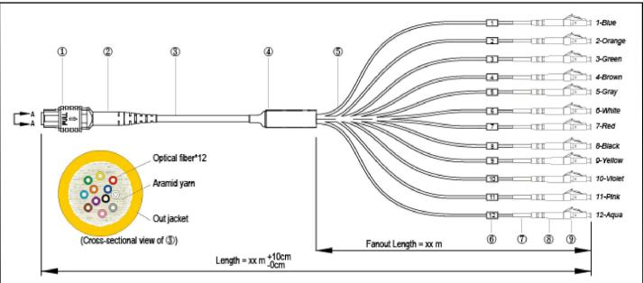
①MPO/MTP Female connector ②Φ3.0mm Boot ③Φ3.0mm – 12 Fibers Mini cable ④Fanout kit ⑤Φ2.0mm Fiber cable
