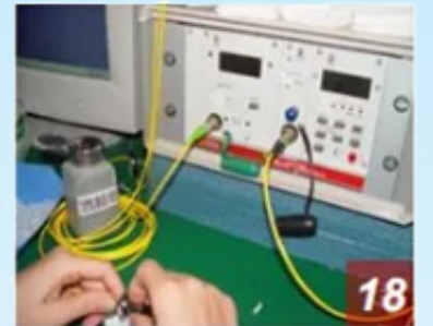
I.L & R.L inspection
